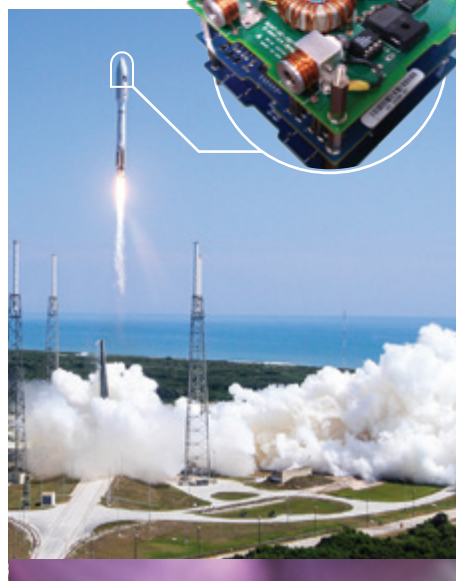
This micro-cathode arc thruster was launched into space in 2015 and used to maneuver a 1.5U CubeSat called BRICSat-P.
