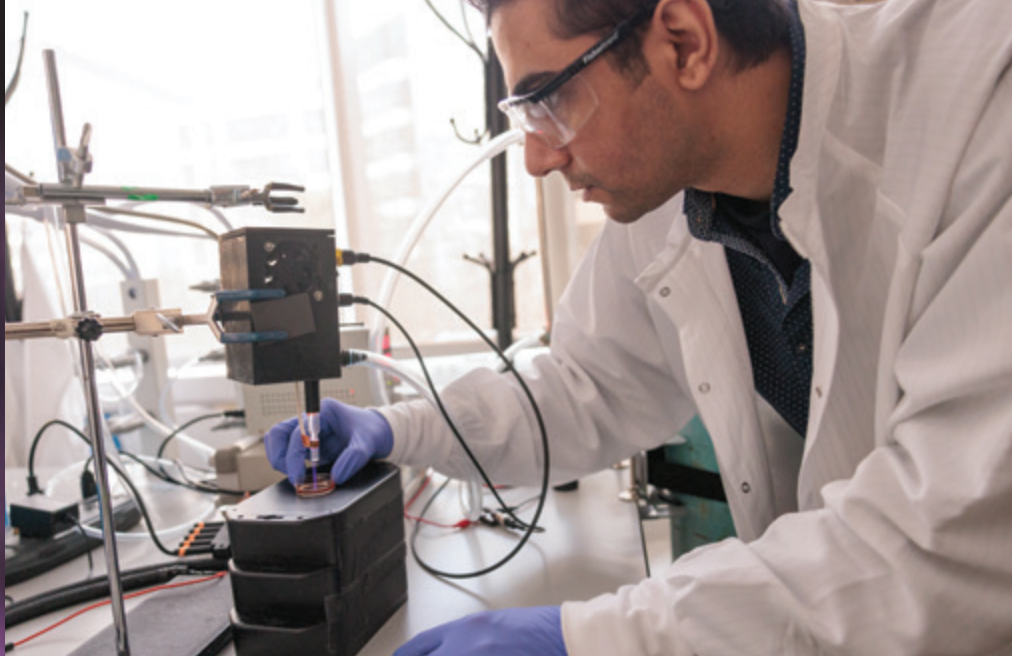
Graduate student Vikas Soni blasts cancer cells in a Petri dish with a jet of cold plasma. After 30 minutes, the cancer cells shrivel up and die.
