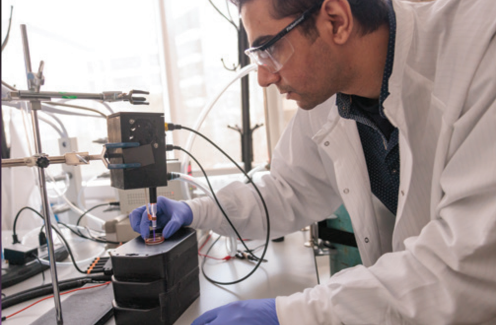
Graduate student Vikas Soni blasts cancer cells in a Petri dish with a jet of cold plasma. After 30 minutes, the cancer cells shrivel up and die.
